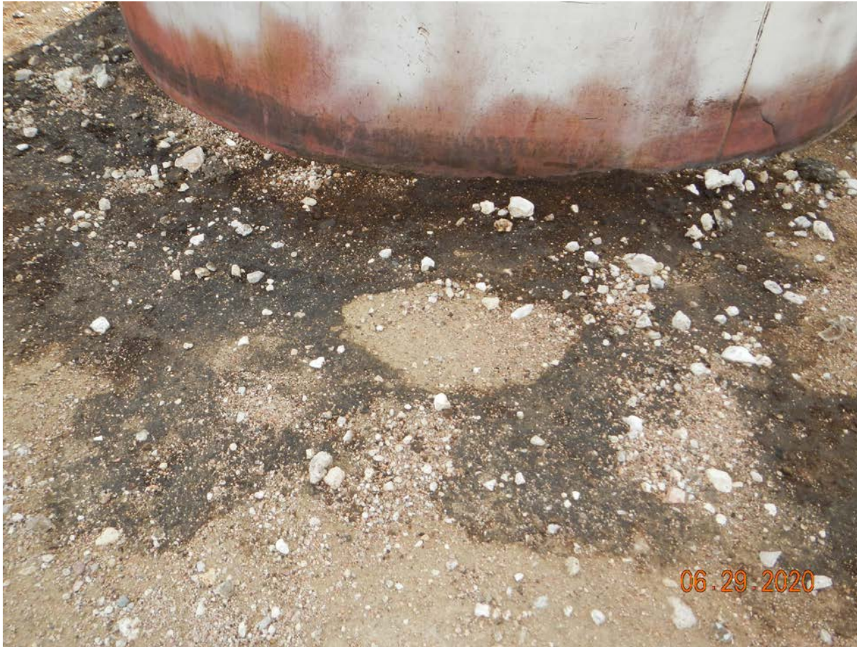
Photo # 6 – East side of tank battery oil stained soil around produced water tank
