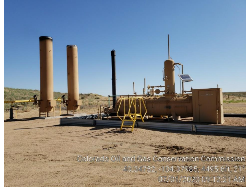
Photo #2 Separator & ECD's
