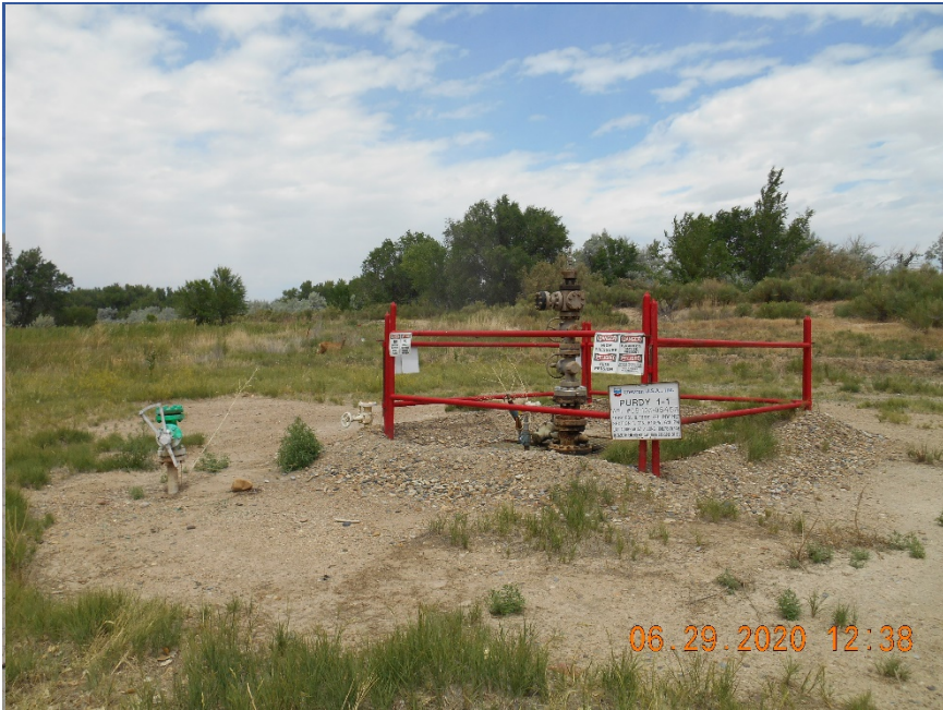
Injection wellhead. Temporarily Abandoned.
