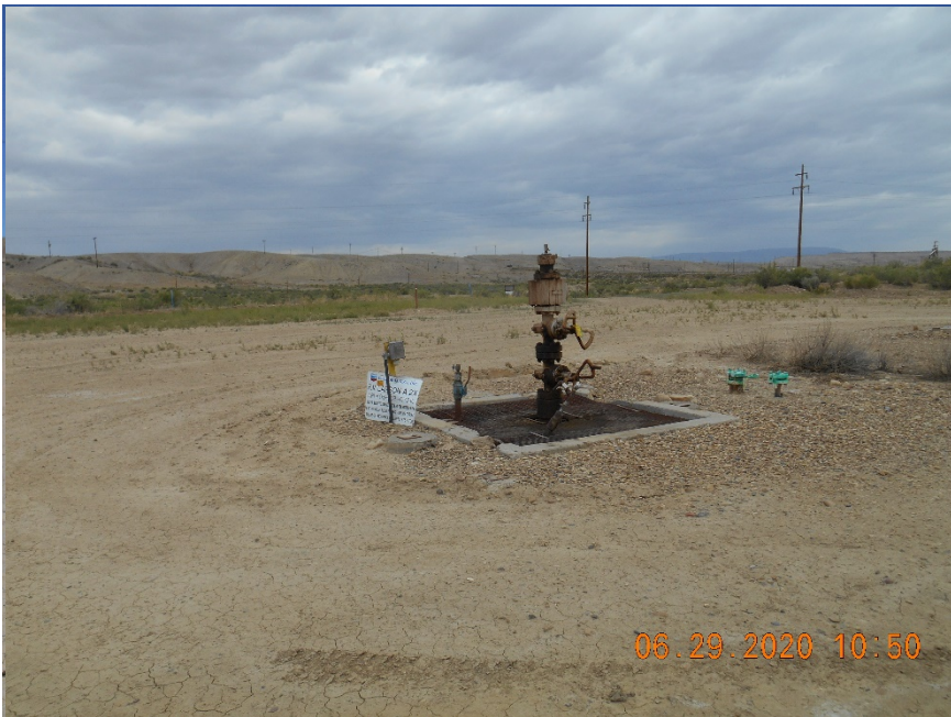
Injection wellhead. Temporarily Abandoned
