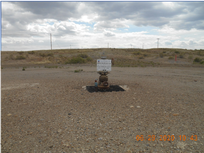
Injection wellhead. Temporarily Abandoned
