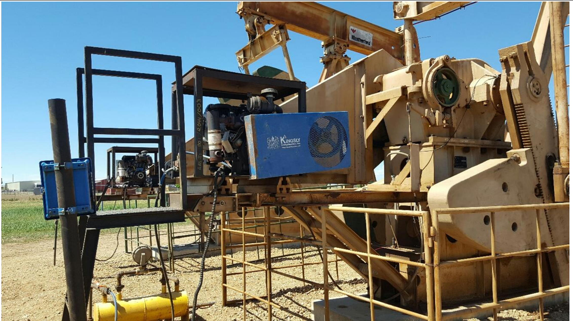
Figure #1 Pulley guard has been installed.
