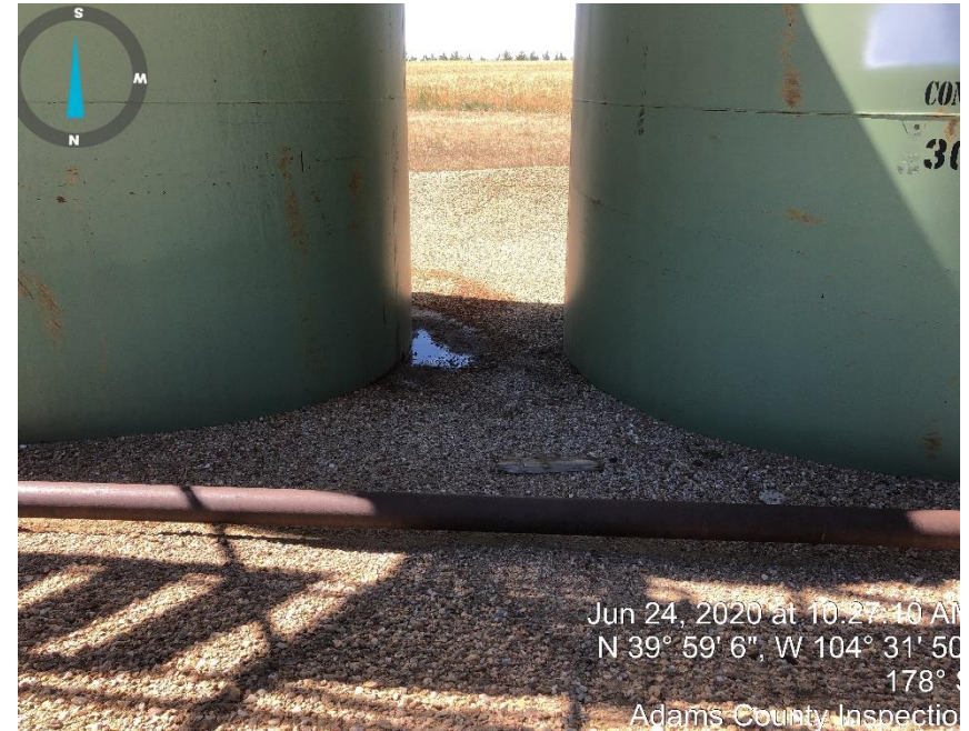
Photo #2 Leak in Condensate tank
