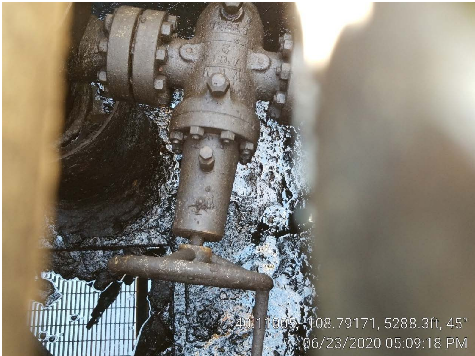
Photo 2. Casing valve.
