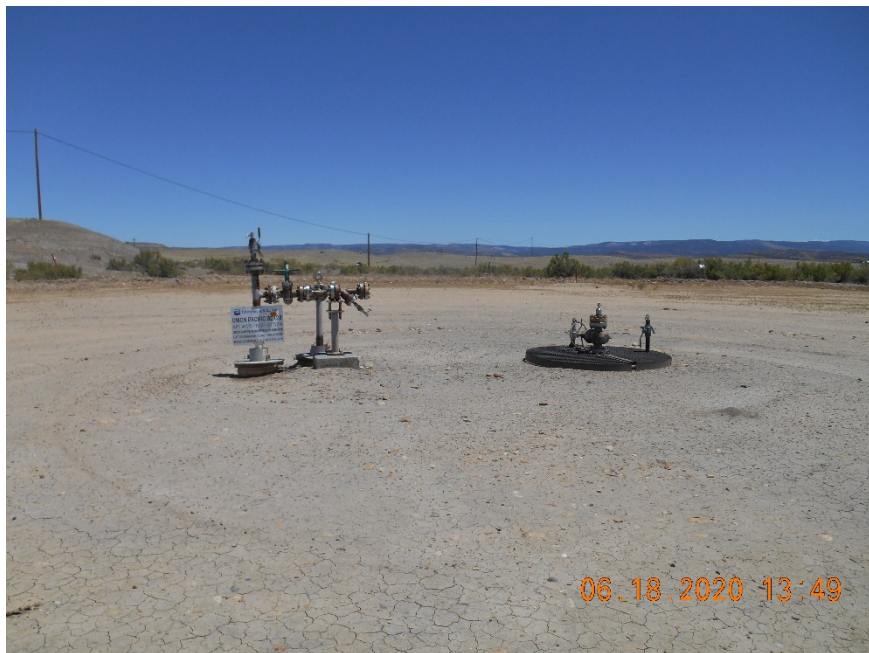
Injection wellhead. Temporarily Abandoned.
