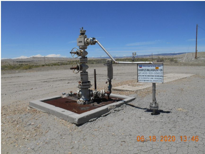
Injection wellhead
