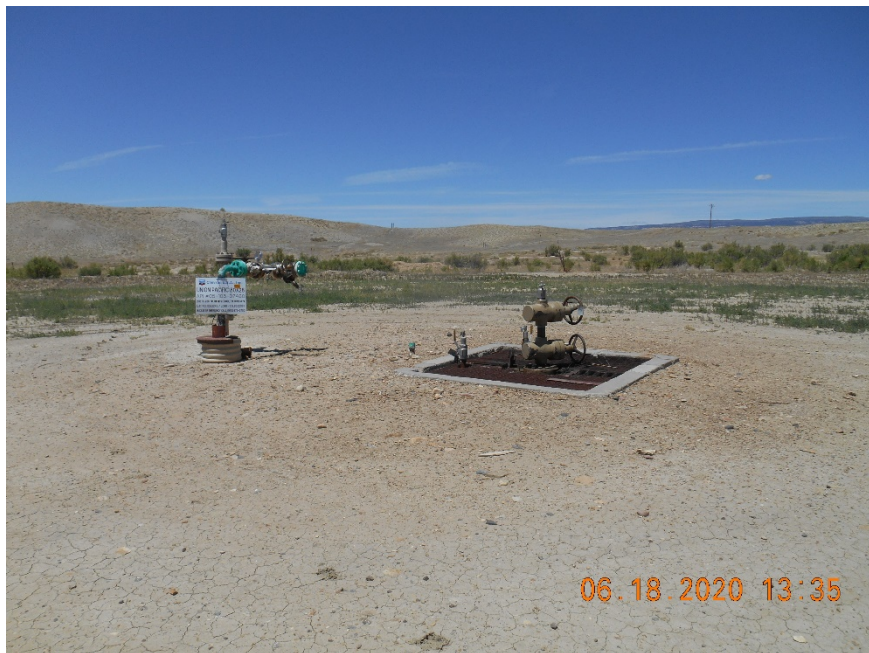
Injection wellhead. Temporarily Abandoned.
