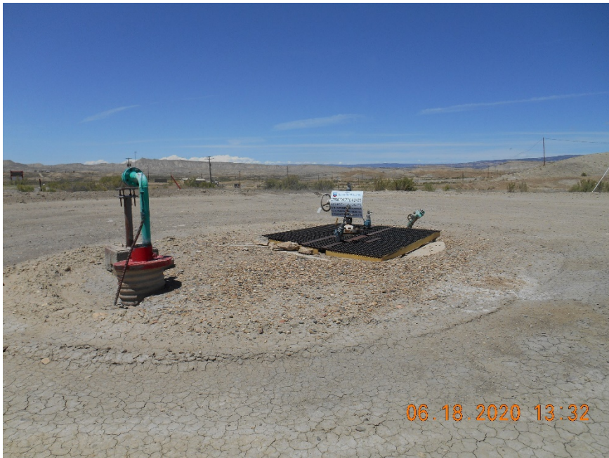
Injection wellhead. Temporarily Abandoned.
