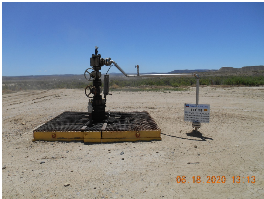
Injection wellhead
