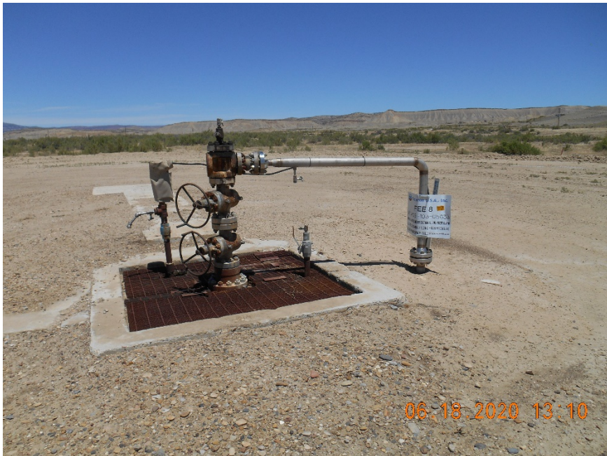
Injection wellhead
