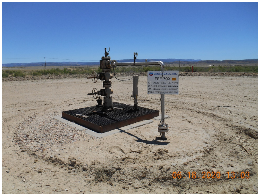
Injection wellhead
