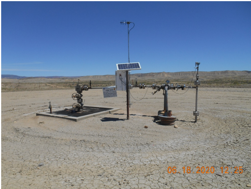
Injection wellhead
