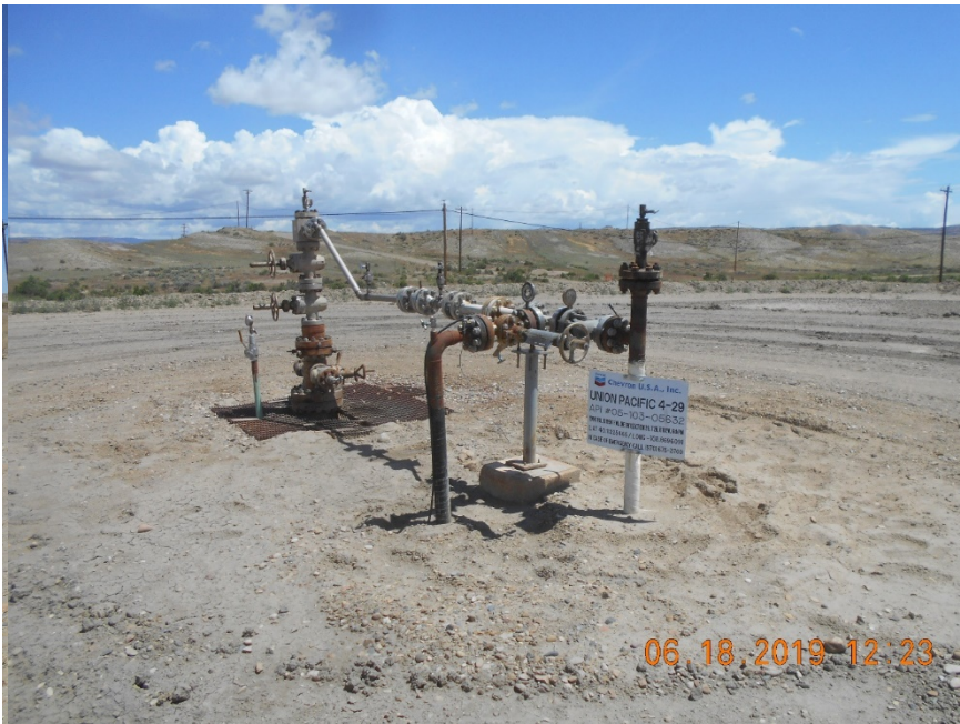
Injection wellhead
