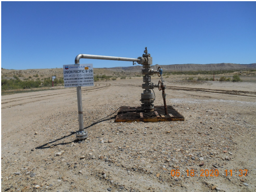
Injection wellhead
