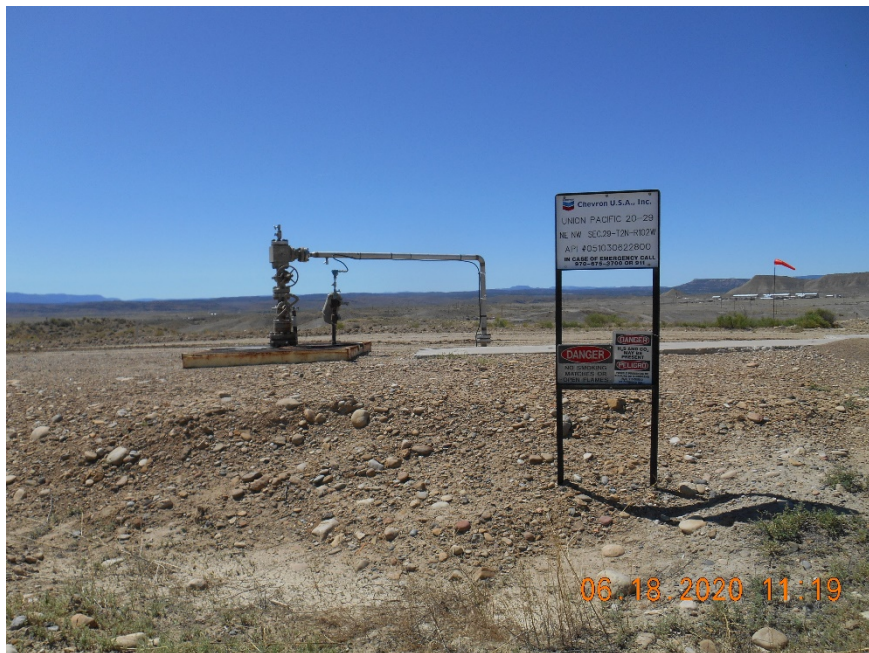
Injection wellhead
