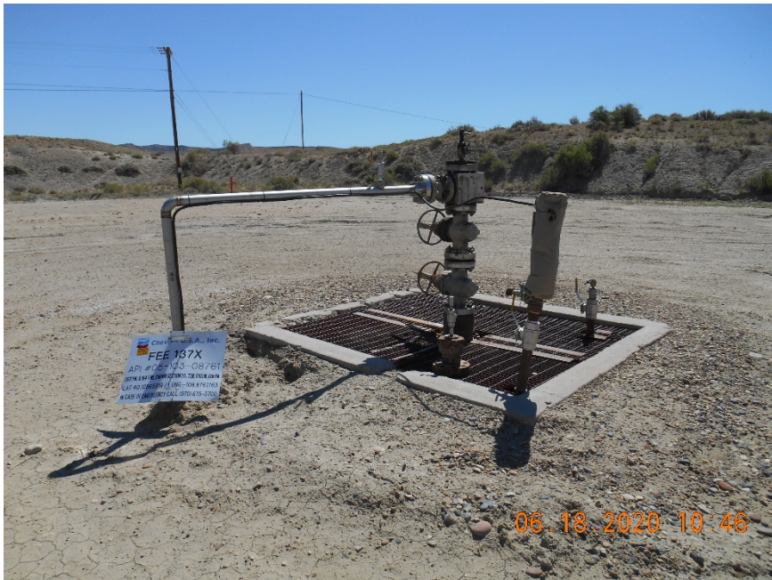
Injection wellhead
