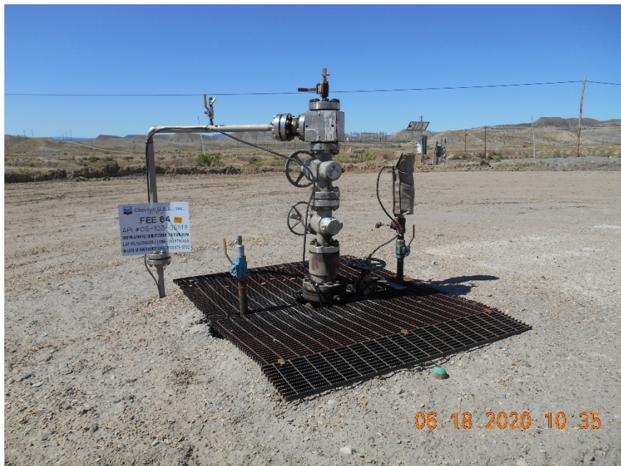
Injection wellhead
