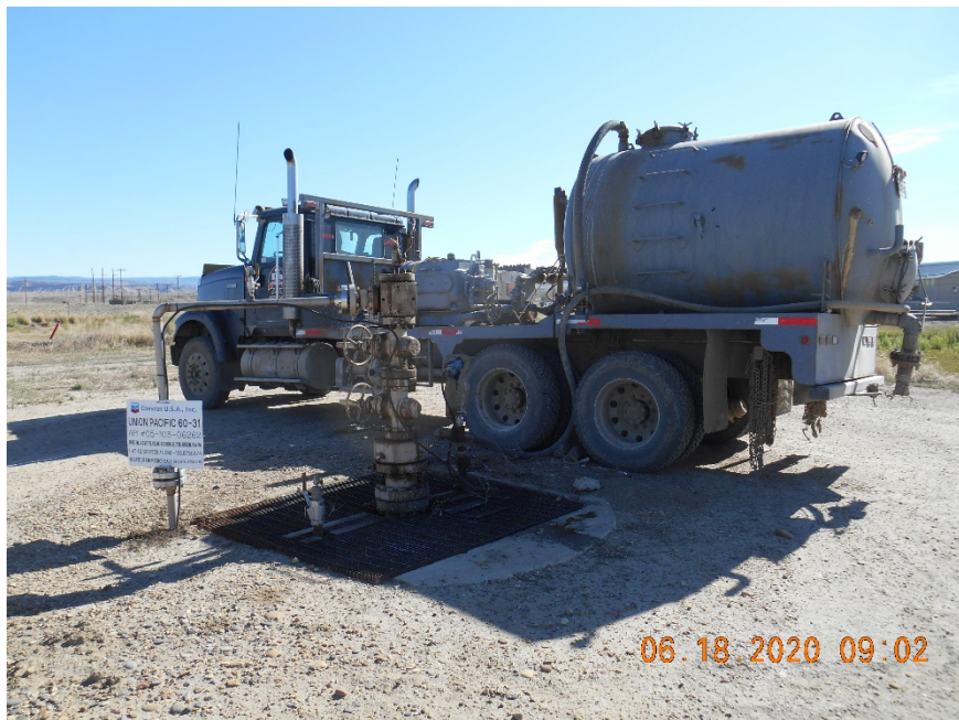
Injection wellhead
