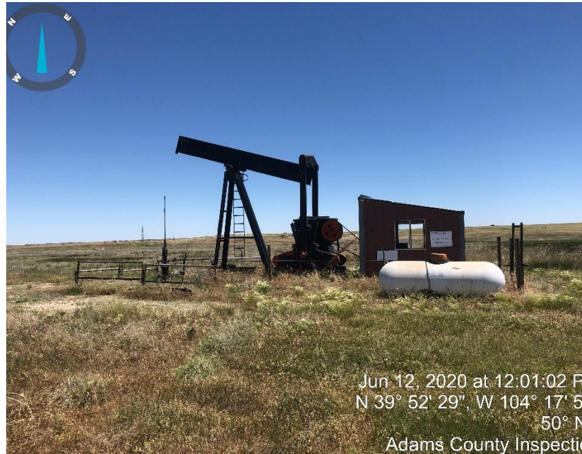
Photo #1 Pump Jack
