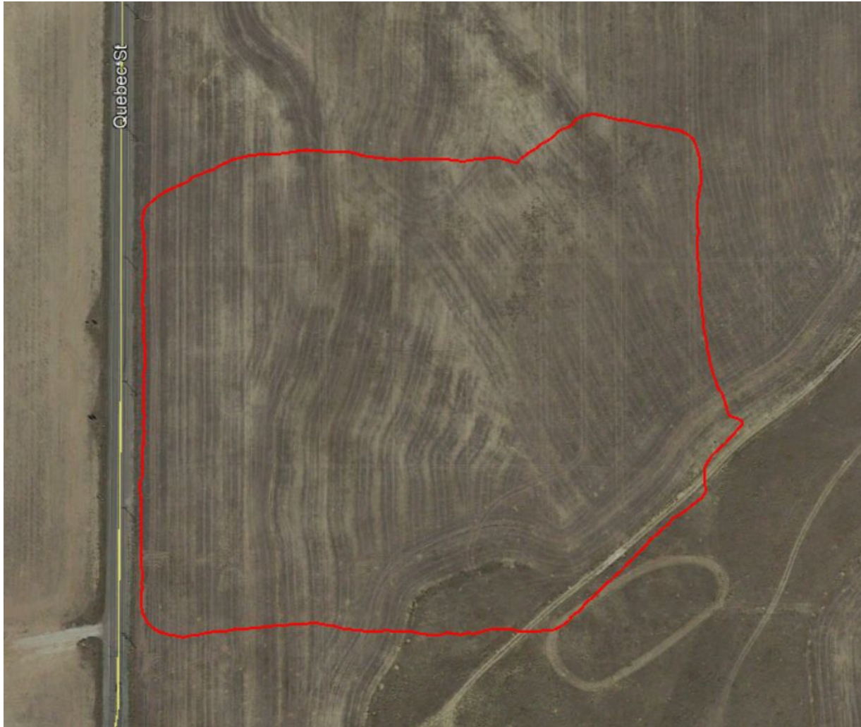
Photo 8. Google Earth aerial imagery taken 9/12/2019. COGCC mapped the outer disturbance area (15.49 acres) using a Trimble Juno 3B handheld device (red line).
