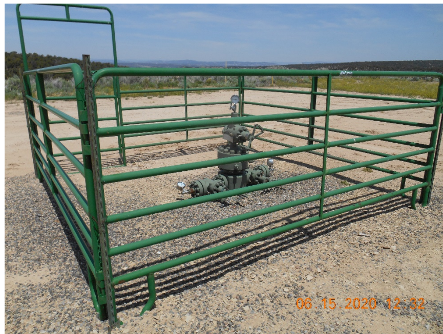
Injection Wellhead Temporarily Abandoned
