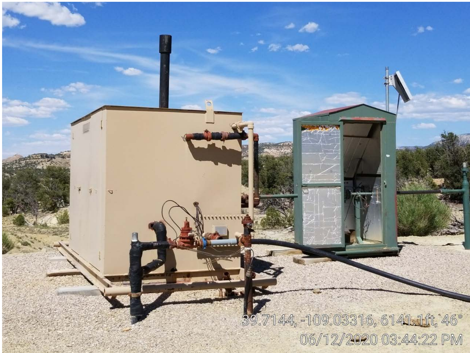
Photo 2. Separator & meter building.
