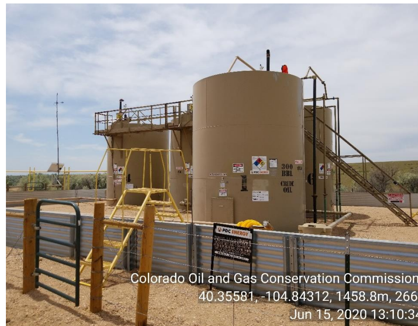
Photo 12: Tank battery
