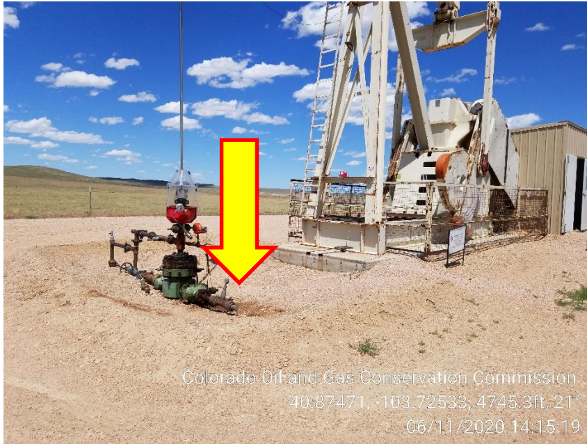
Photo 1 – Pumping Unit, Stained Soil at Wellhead
