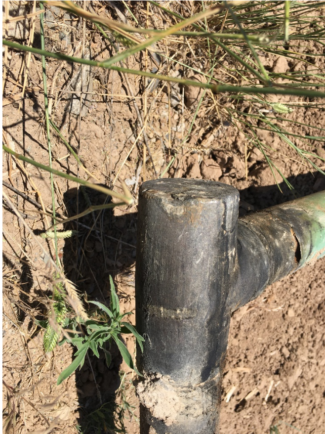
Target tee's showing external corrosion
