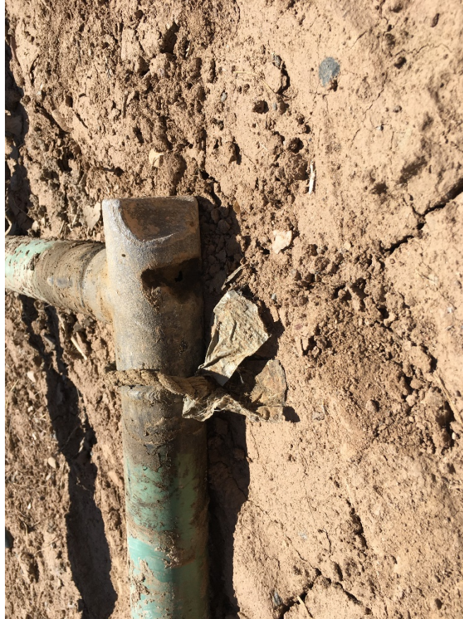
Target tee's showing external corrosion
