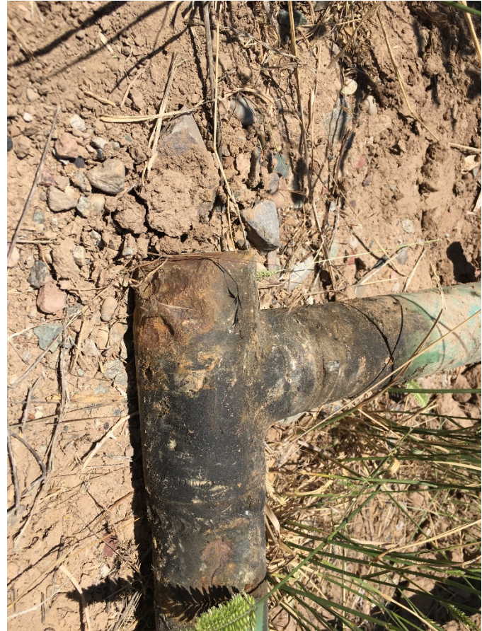
Target tee's showing external corrosion
