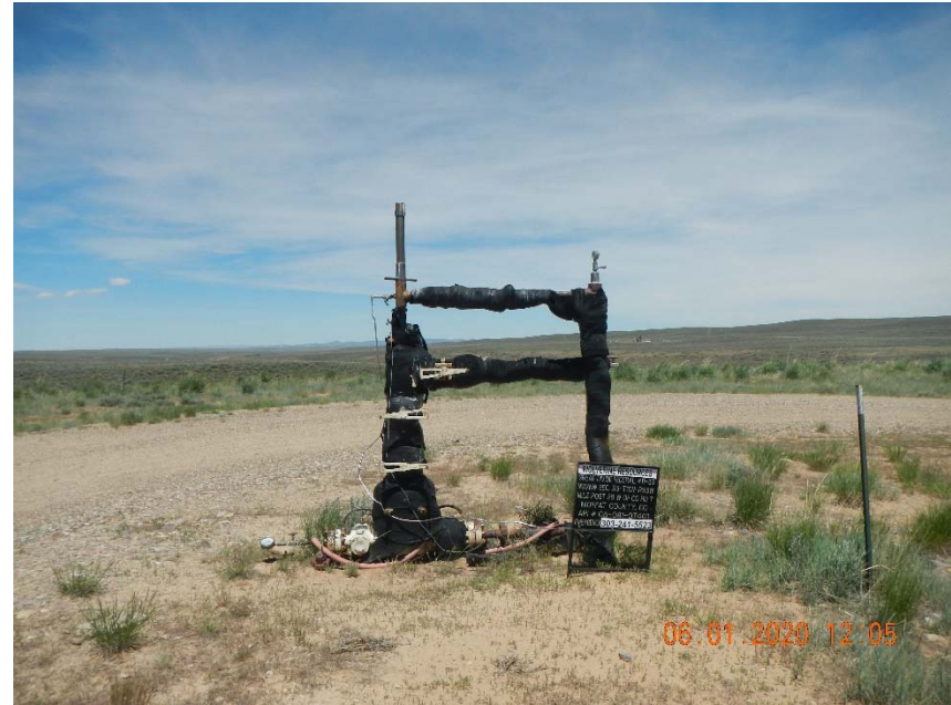
Photo 2. Hissing heard at wellhead.
