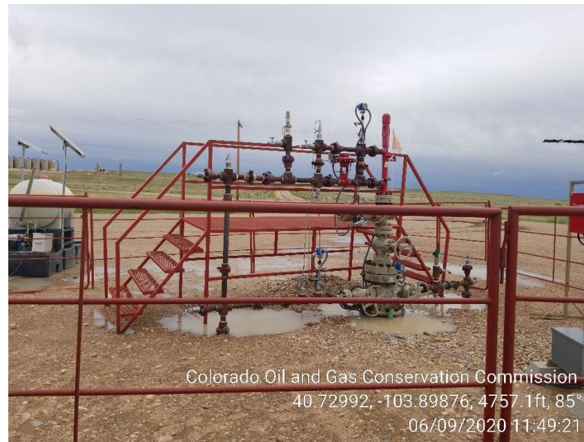
Photo 2 – LD29-78HN, Wellhead Sign missing
