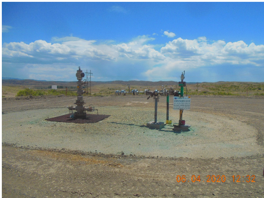
Injection wellhead. Temporarily abandoned.
