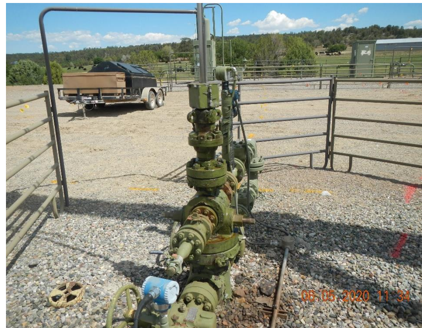
Wellhead is wet with lubricating oil from stuffing box.
