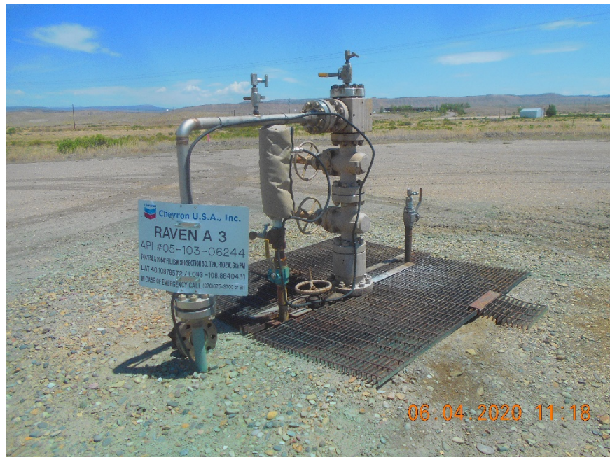
Injection wellhead.
