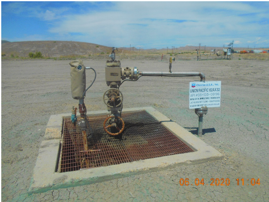
Injection wellhead.
