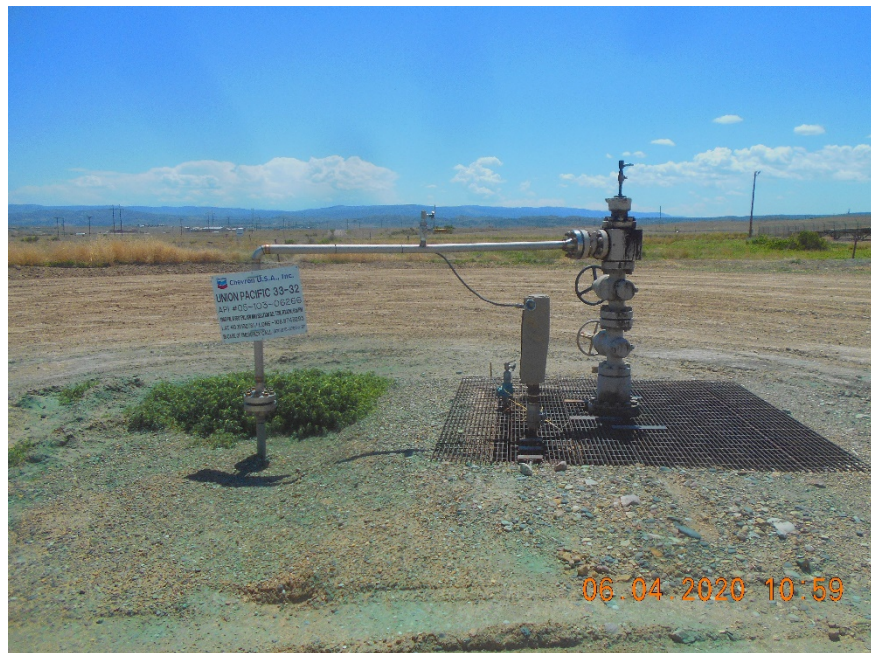
Injection wellhead.
