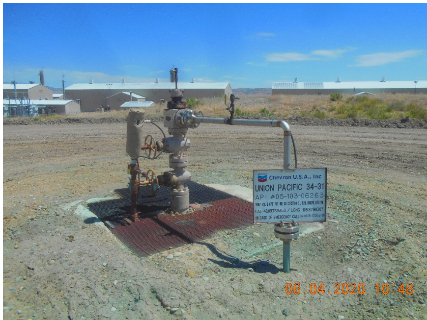
Injection wellhead.
