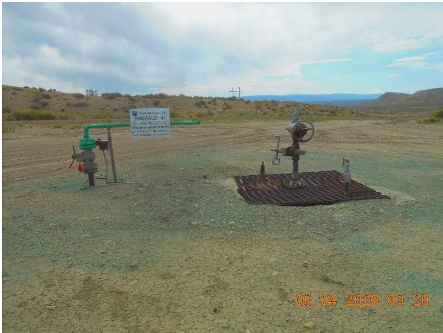
Injection wellhead. Temporarily Abandoned
