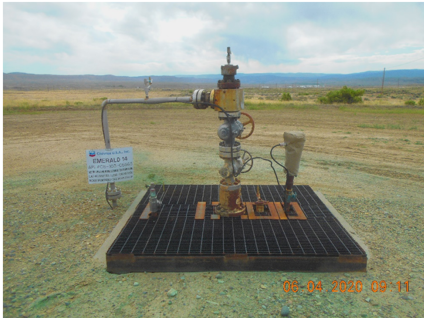
Injection wellhead.
