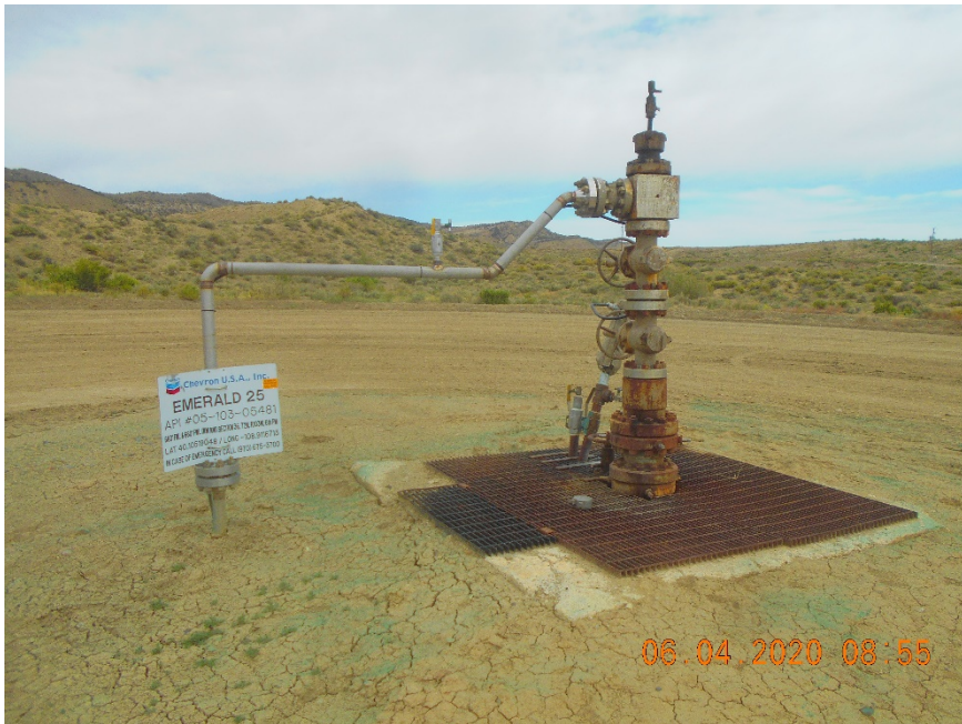
Injection wellhead.
