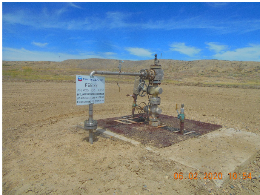
Injection wellhead.
