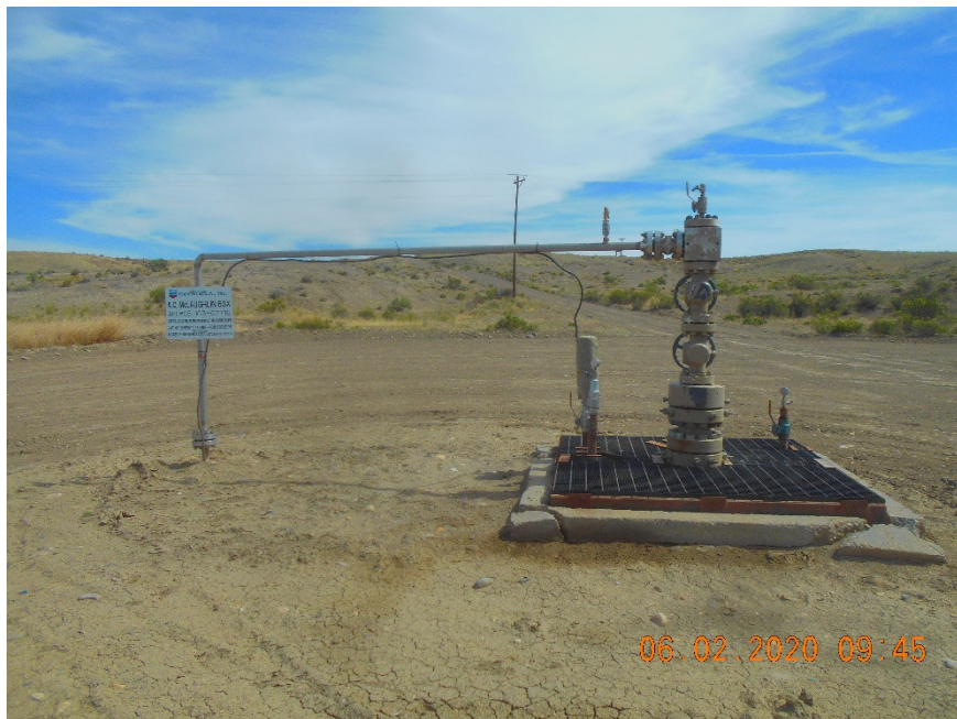
Injection wellhead
