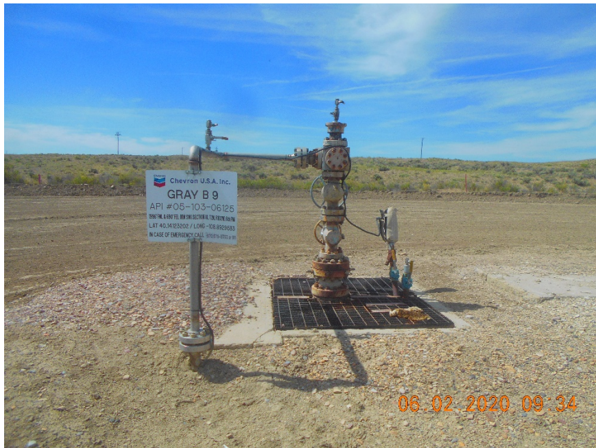
Injection wellhead
