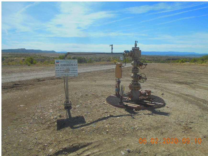
Injection wellhead
