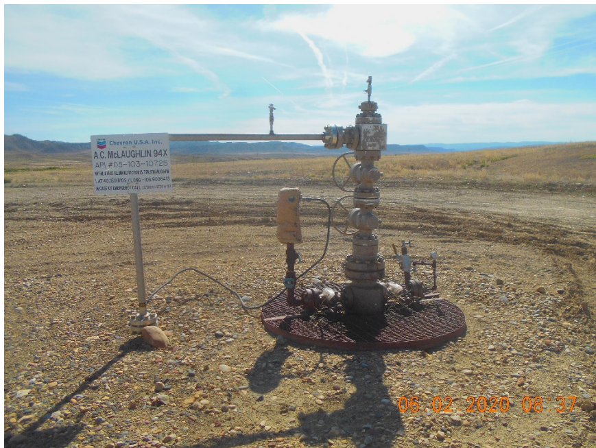
Injection wellhead
