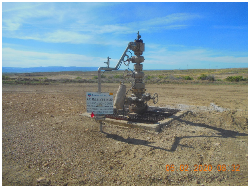
Injection wellhead
