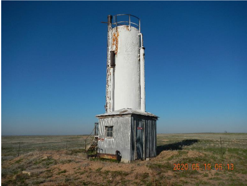
Photo 3: Heater treater and shed.
