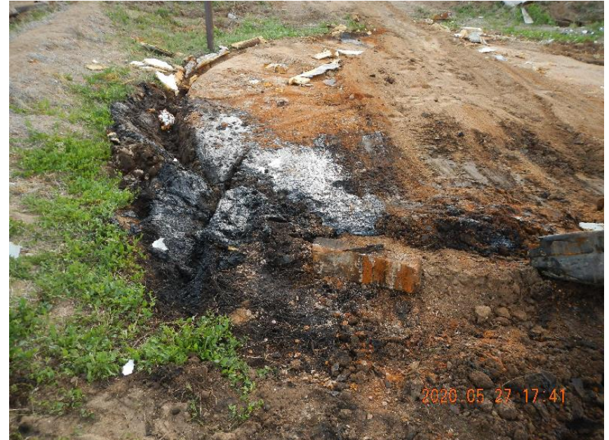
Photo 20: Impacted soil that was under production tank 3 in SE corner of tank battery.
