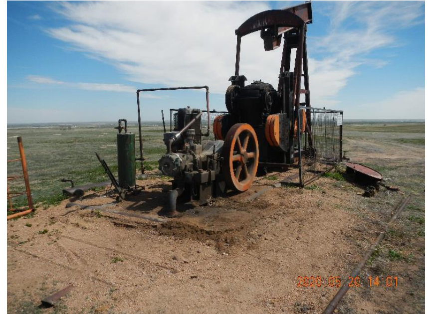
Photo 6: Pumping unit after shed removed.
