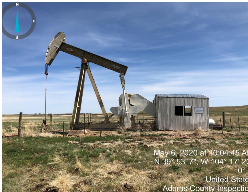
Photo#3 Wellhead and Pumpjack
