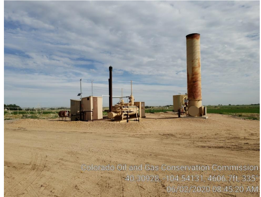
Photo #4 Separator, ECD & Meter Run
